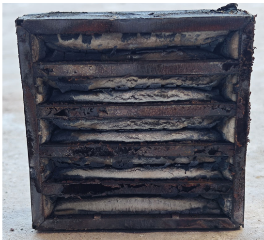
DFG (Unexposed Side) - 30 min into Fire Resistance Test
